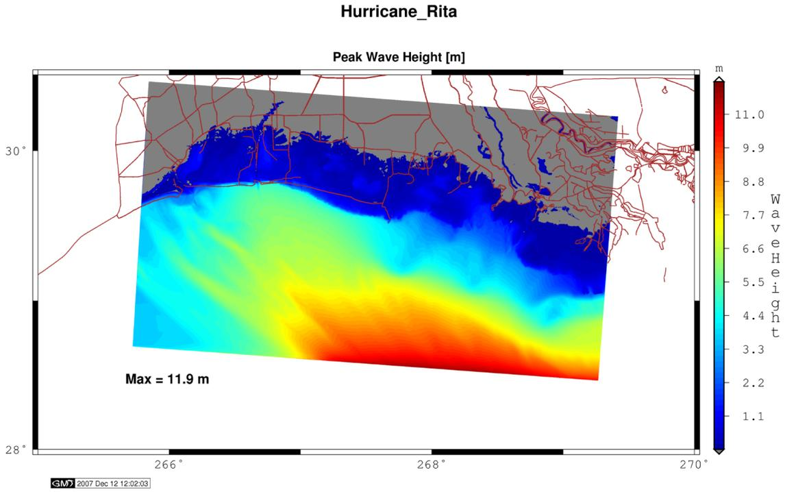
Figure 279: Maximum significant wave height during Hurricane Rita validation (West grid).
